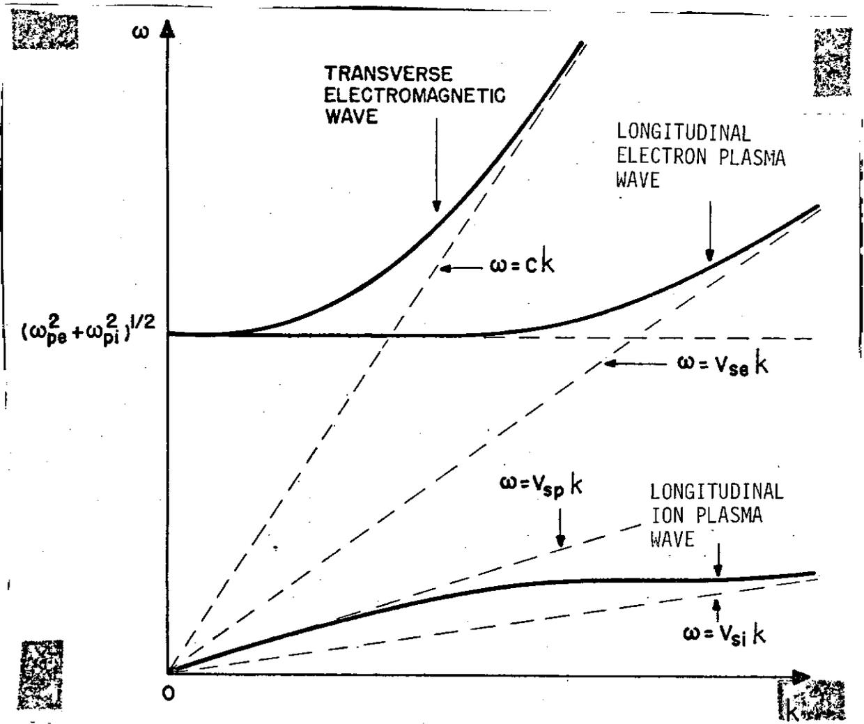
Fig. 2 - Dispersion relation for the three modes of wave propagation in a warm isotropic fully ionized plasma.
