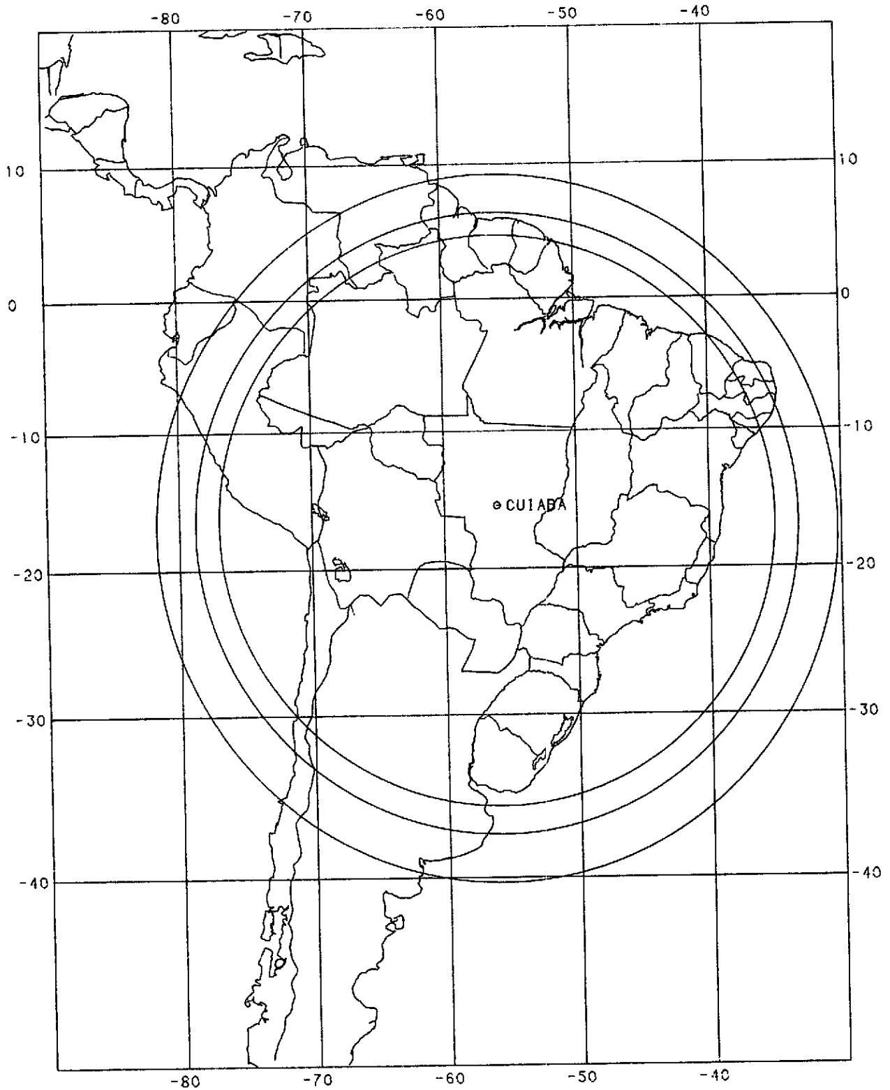
Fig. 10 - Visibility circles for the Remote Sensing Satellite from the Cuiabá earth station with minimum elevation angles of 0^{\circ} , 30^{\circ} , and 5^{\circ} .
