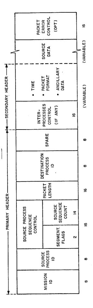
INTERPROCESSES CONTROL: DEFINES THE CONTROL BETWEEN THE TWO PROCESSES IN COMMUNICATION , IF NEEDED. DESTINATION PROCESS ID DEFINES THE PROCESS THAT RECEIVES THE PACKET SOURCE PROCESS ID DEFINES THE PROCESS THAT CREATES THE PACKET OTHERWISE IT WOULD NOT OPERATE.
