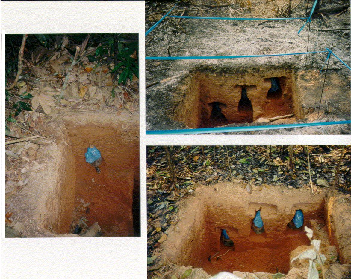
Figure 2 – The 1999 trenches with the zero-tension lysimeters: pristine forest G (left), slashed and burned area D (upper) and burned litter F (right).
