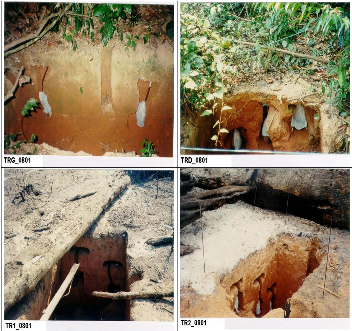
Figure 3 – The 2001 trenches with the zero tension lysimeters: pristine forest G (TRG), regrowth of the 1999 slashed and burned area E (TRD), and inside the 2001 slashed and burned area F (TR1 and TR2).
