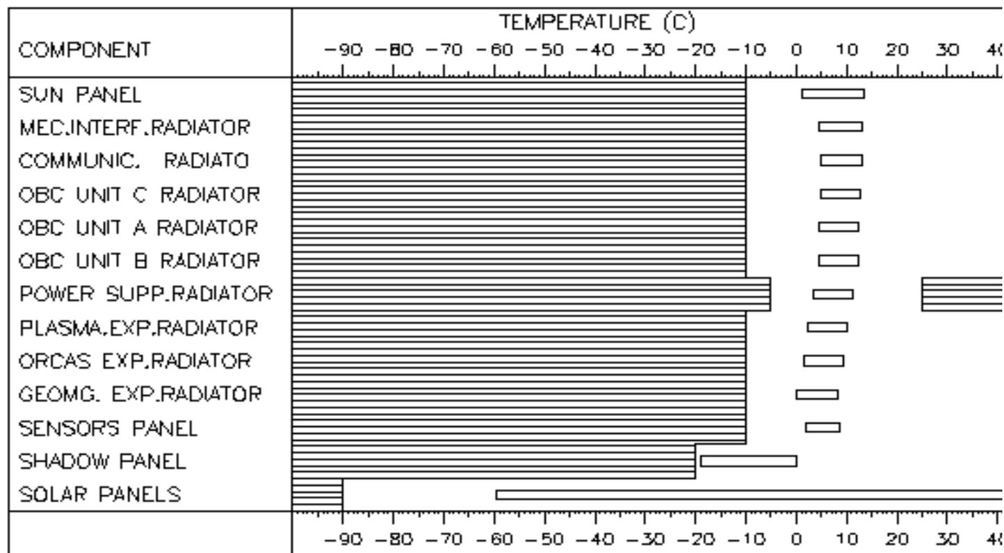
**Fig. 4 : Predicted Temperature For The Operation Phase.**
