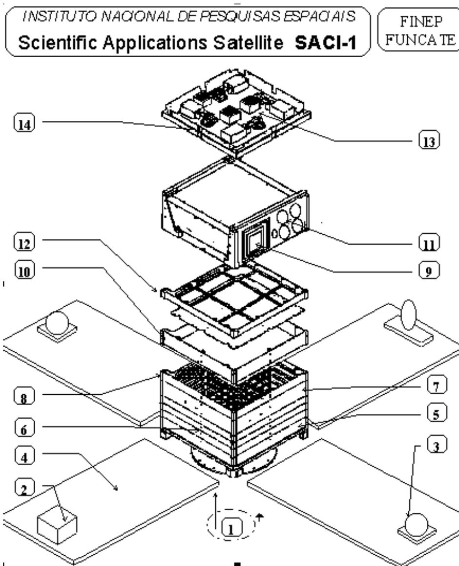
**1 - Solar Panels Sun Face 2 - Magnetometer Sensor**
