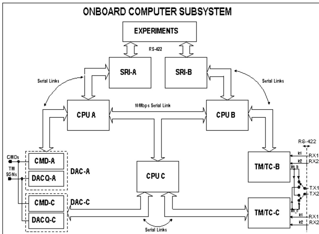
**Fig. 3: On-board Computer Subsystem Block Diagram.**
