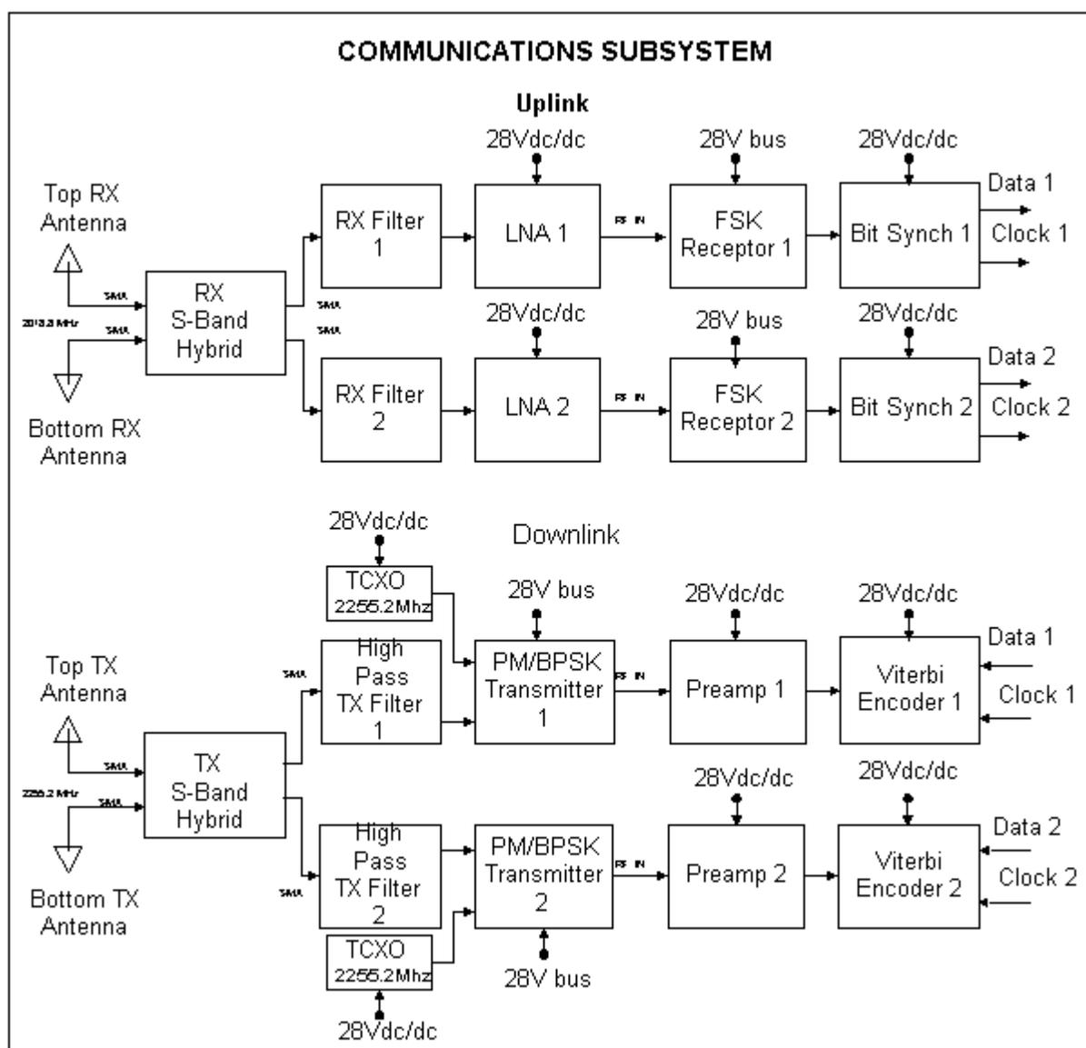
**Fig. 6: Communication Subsystem Block Diagram.**
