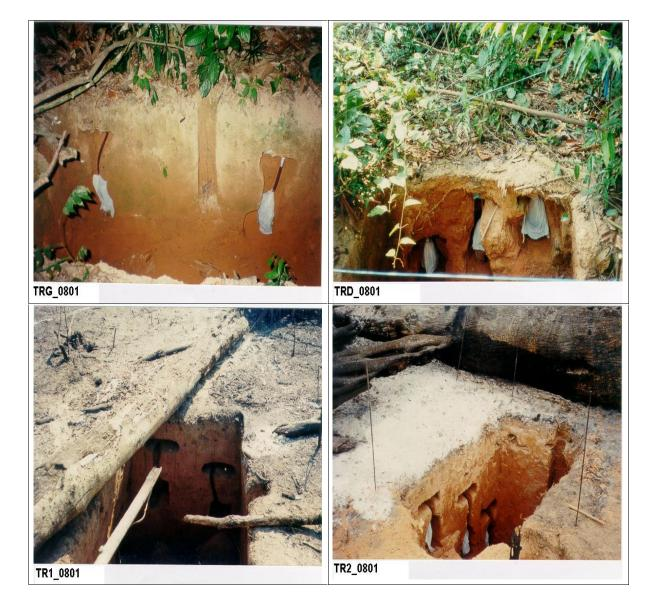
Figure 3 – The 2001 trenches with the zero tension lysimeters: pristine forest G (TRG), regrowth of the 1999 slashed and burned area E (TRD), and inside the 2001 slashed and burned area F (TR1 and TR2).
