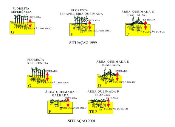
Figure 1 – Configuration of the zero-tension lysimeters in the trenches.
