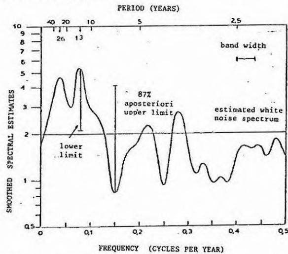
Fig. 1 - Smoothed spectral estimates for Fortaleza annual rainfall time series (1849-1978). The band width of 0.037 was chosen so as to discriminate the frequencies of 1/13 and 1/26.
