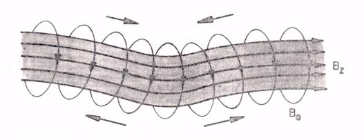
Fig. 15 - The increased tension of a longitudinal magnetic field, applied inside the column, inhibits the kink instability.
