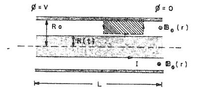
Fig. 8 - Sheamatic representation of the closed loop, for application of Faraday's law, with the inner side lying on the interface and moving inwards with it.
