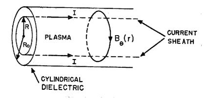
Fig. 6 - Plasma column of infinite conductivity, inside a hollow cylindrical dielectric, with a current sheath on its surface.
