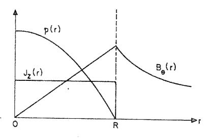
Fig.3 - Radial dependence of the azimuthal magnetic induction  $B_{\Theta}(r)$ and plasma pressure p(r) in a cylindrical plasma column with a constant current density  $J_z(r)$ . The radius of the column is R.
