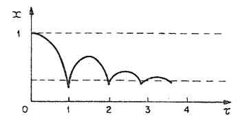
Fig. 10 - Normalized radius of the plasma column as a function of the normalized time, illustrating the phenomenon of bouncing.
