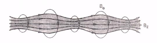
Fig. 13 - A longitudinal magnetic flux density  $B_z$  can be used to inhibit the sausage instability.
