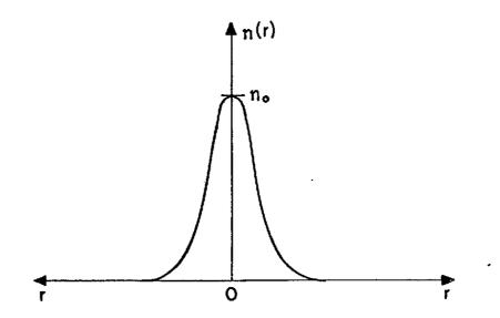
Fig. 5 - The Bennett distribution of the number density, n(r), of the particles in an equilibrium pinched plasma column.
