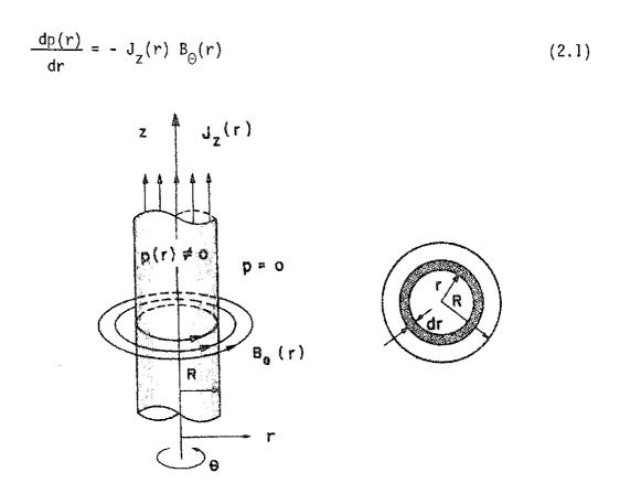
Fig. 2 - Schematic diagram illustrating the various parameters relevant to the study of the equilibrium longitudinal pinch configuration.
