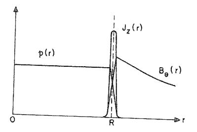
Fig. 4 - Radial dependence of the azimuthal magnetic induction,  $B_{\Theta}(r)$ , and plasma pressure, p(r), in a cylindrical plasma column with a current restricted to a very thin layer on the surface of the column.
