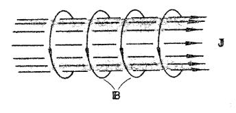
Fig. 1 - Pinch configuration in which a magnetoplasma is confined by azimuthal magnetic fields generated by axial currents flowing along the plasma column.
