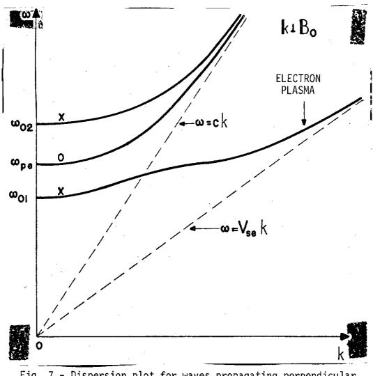
Fig. 7 - Dispersion plot for waves propagating perpendicular to  $B_{\sim 0}$  in a warm electron gas.
