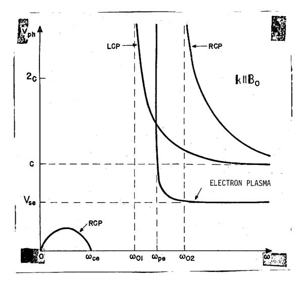
Fig.4 - Phase velocity, as a function of frequency. for waves propagating in the direction of  $B_{\sim 0}$  in a warm electron gas.
