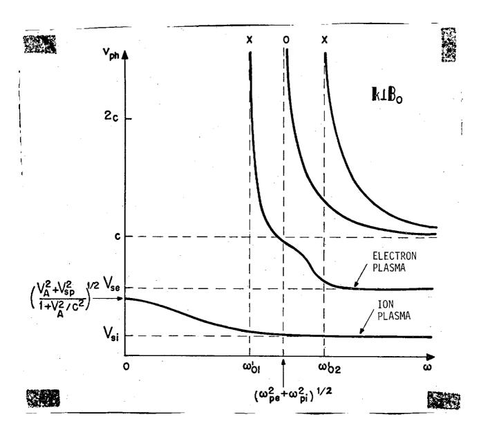
Fig. 10 - Phase velocity as a function of frequency for waves propagating in a direction normal to the magnetic field in a warm fully ionized magnetoplasma.
