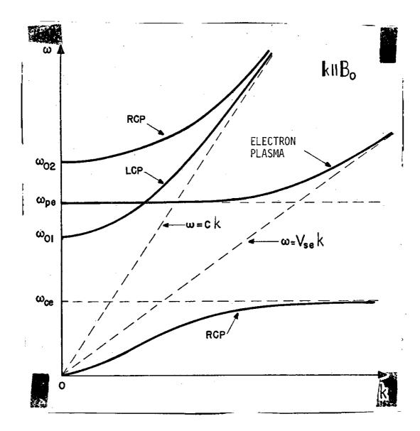
Fig. 5 - Dispersion plot for waves propagating parallel to  $\underset{\sim 0}{B}$  in a warm electron gas.
