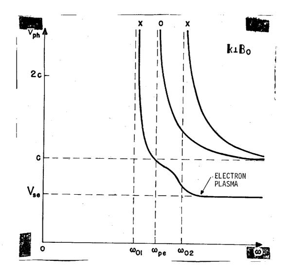
Fig. 6 - Phase velocity as a function of frequency for waves propagating perpendicular to  $B_{\sim 0}$  in a warm electron gas.
