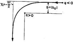
Fig. 7 - Scattering in a Coulomb potential field for a deflection angle,  $\chi$ , of 90 $^{\rm O}$ .
