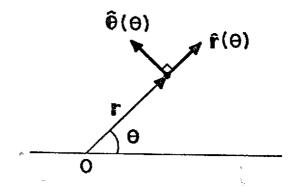
Fig. 5 - Polar coordinates (r,  $\Theta$ ), showing that the directions of the unit vectors  $\hat{r}$  and  $\hat{\Theta}$  depend on  $\Theta$ .
