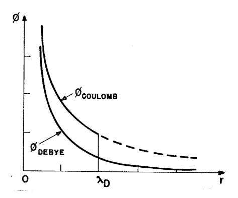
Fig. 9 - The approximation used to obtain  $\sigma_t = \pi \lambda_D^2$  consists in assuming that for  $r < \lambda_D$  the shielding effect is completely omitted and the particles interact according to the Coulomb potential, whereas for  $r > \lambda_D$  the shielding of the target particle is assumed to be complete and there is no interaction.
