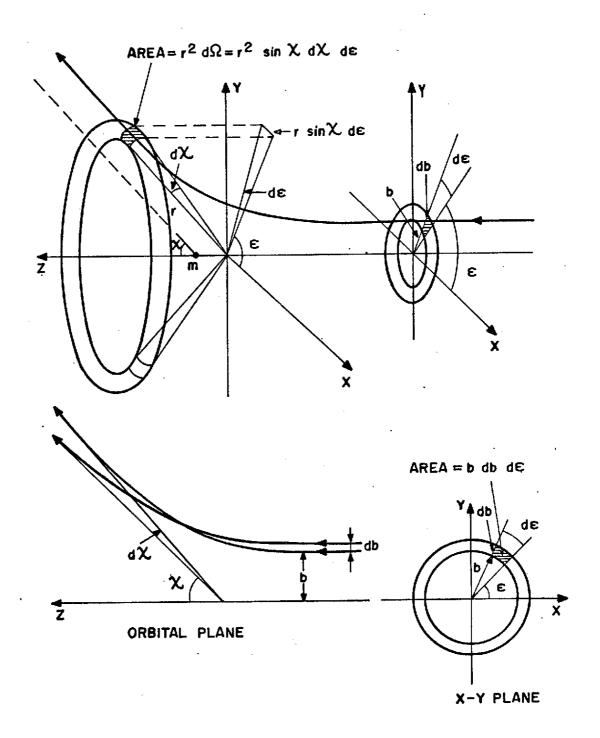
Fig. 8 - Scattering in a central field of force.
