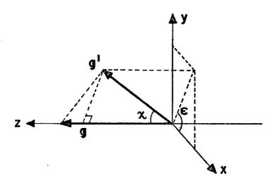
Fig. 3 - Relationship between the relative velocities  $\underline{g}$  and  $\underline{g}'$ , in a Cartesian coordinate system for which  $\underline{g} = g \ \widehat{z}$ . The angle  $\varepsilon$  defines the relative orientation of the plane containing the particle trajectory.
