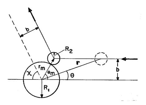
Fig. 6 - Collision between two perfectly elastic impenetrable spheres.
