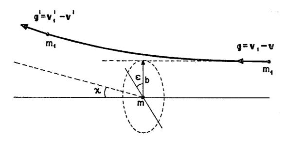
Fig. 2 - Geometry of a collision between a particle of mass m and velocity  $\underline{v}$ , and a particle of mass  $m_1$  and velocity  $\underline{v}_1$ , viewed from a coordinate system in which the first particle is at rest.
