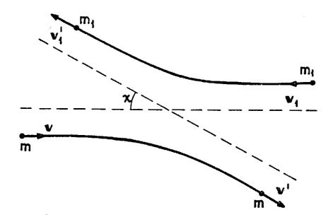
Fig. 1 - Binary interaction of two particles of mass m and  $m_1$ , with velocities  $\underline{v}$  and  $\underline{v}_1$ , respectively, as viewed from the laboratory system.
