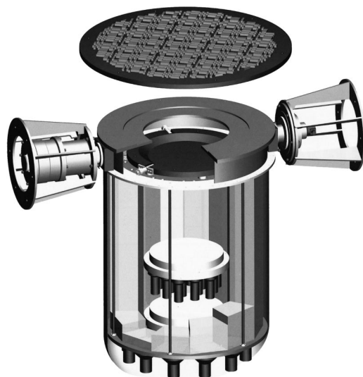
FIG. 1. A general view of the imaging system of the MASCO experiment with the distance to the mask not to scale. The detector system is placed inside a pressure vessel and the distance from the mask to the detector surface is 3.05 m.
