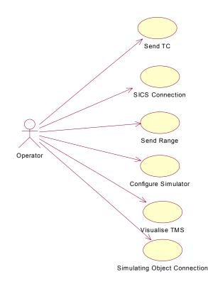
Figure 4.1 – The Use Case Diagram – Subsystem Simulator
