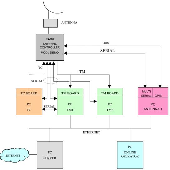
Figure 1: SACI Ground System Architecture
